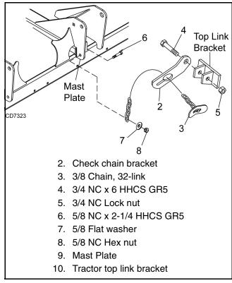
Figure 36. Optional Check Chain Assembly
